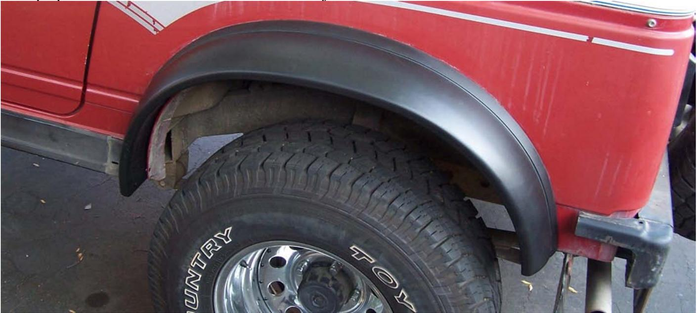
**Step 3** - Align the Scribe Line on the flare to the *Center Outer Hole* of the bracket. We suggest you find the scribe line first. It's underneath the flare at the very top tangent point. Mark it with the white out pen so it's easier to see when in place. It must be aligned with the outermost hole in the center of the bracket. Refer to the **step 1b photo**. Hint: Find the 2 holes close together on the highest point of the bracket. The outside one is the one you will use for marking.
