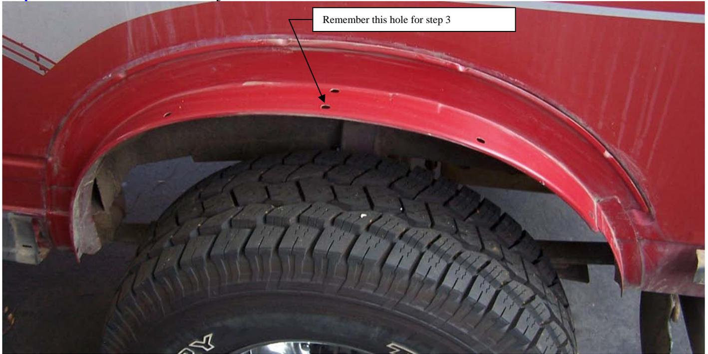
**Step 1c – If applicable, remove front & rear Rocker Cover End Caps as well as rear Bumper Caps.**
