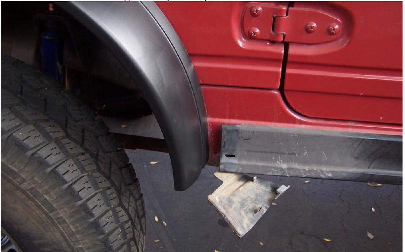
**Step 2** - Slip the MudBusters in place over the factory bracket. Longer two flares go in the rear with the 1-inch hole forward. Shorter flares go in the front with the 1-inch hole to the rear. Place a flare against the fender, an inch or two above the factory bracket and slide it downward. Insure that the plastic tabs under the top lip tuck between the bracket and the fender just like the old flares.
