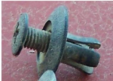
**Tip:** If the rivet screw threads are full of dirt they sometimes won't back out when unscrewing. Some tricks are to pull back on the screw head with a tiny flat blade screwdriver while unscrewing with the Phillips or just pry the entire rivet out with needle nose pliers. We drilled our screw heads off with a 1/4" right angle drill and used new rivets because they hold tighter than the old rivets.
