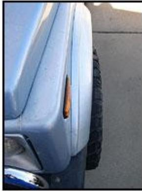
You can see that they are similar, but twice the width of the stock fenders. These photos show how much a set of 31/10.50/15R tires show when mounted on standard 8" rims with 3.75" of back space. Although this installation shows us replacing the 'early' style fenders, they are also a direct replacement for the newer steel fenders, you just use the plastic clips (included) instead of the 10mm bolts.
