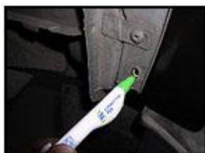
The holes for the retainer clips are not drilled at the factory, just in case your panels are a little out of alignment. Using a white marker (I used a 'white-out' pen) you can mark the holes for drilling. Once the holes are drilled, just drop them
