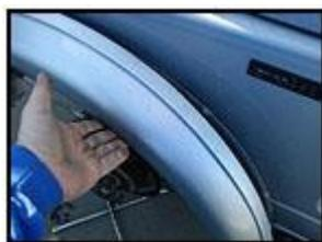
The stock fender lifts off of the body mounted retaining bracket. Look closely at the edge of the fender and you will notice the ridges that hook over the retaining bracket. The new fenders use the same kind of ridges, so set them in place like
