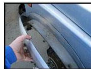
the stock fenders. The front fenders have are not interchangeable (left to right), so make sure you match the the shape to the originals.
